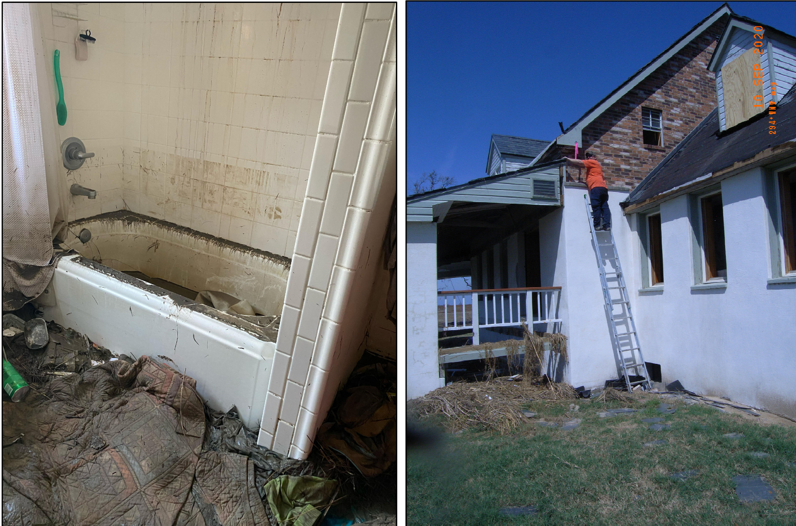
Figure 7. (a) Storm surge high water mark above a bathtub on the second story of a home in the Oak Grove neighborhood of Creole, Louisiana. (b) USGS survey team extrapolating the high water mark to the outside of the home to survey its elevation of 17.1 ft above ground level. Images courtesy of the NWS and USGS.
